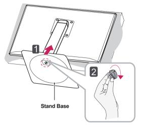
Applying excessive force when tightening screws may cause damage to the monitor. Damage caused in this way will not be cov-ered by the product warranty.
